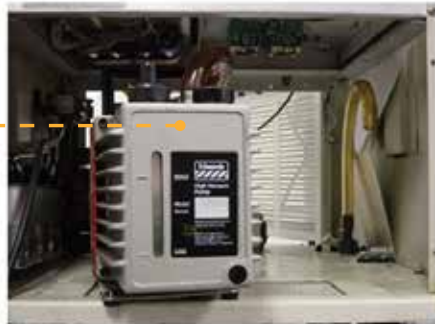
Step 3: Pull the mechanical pump to the edge of the MGA 1200
