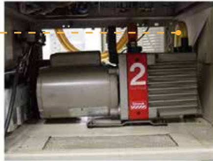
Step 2: Take off oil vapor tube
