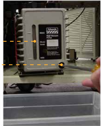
Step 4: Remove oil plug
