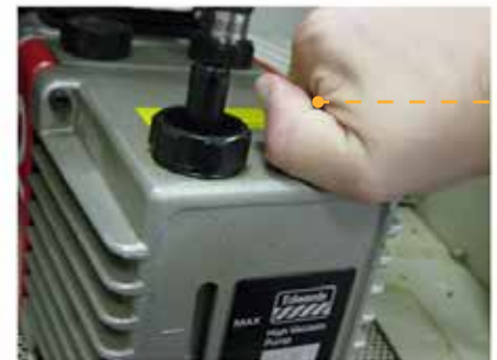
Step 5: Remove oil cap and fill with new oil halfway up.
