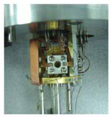
Step 2: Pull off the filament leads from the pins with needle nose, but not all of them just the ones you need to, from pins 3, 6, and 9
