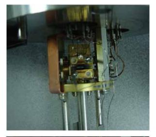
Step 4: Make sure the two insulators are in place (the shoulders in it's notch).
