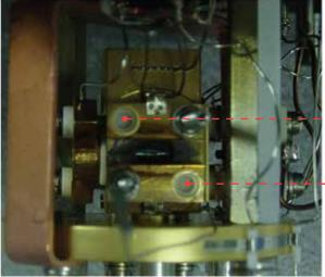
The Insulators shoulders slide right in here, the Filament has the same fittings for the Insulators shoulders
